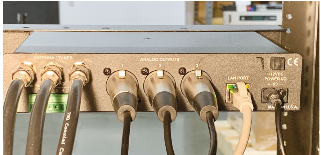
Above The 677's rear panel provides discrete RF inputs and audio outputs for each tuner.
