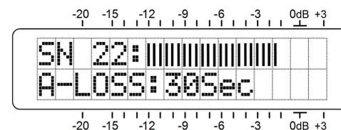
FM receivers generate a good deal of white noise (hiss) in the absence of a carrier. For this reason, the INOmni 636 audio-loss alarm function is really valid only for an unmodulated carrier... it may or may not be triggered if the weather broadcast transmitter goes off the air. A transmitter failure will give you a low signal alarm, however.
