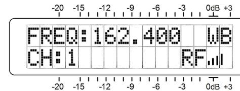
The first line of the LCD display shows the tuned frequency **FREQ:** in MHz, along with a fixed notation that you are indeed tuning the Weather Band, **WB**.
