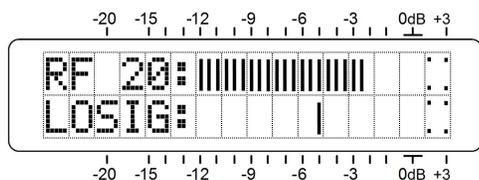
The lower LCD scale is labeled LOSIG: and has a single tic mark off to the right. Push the knob and LOSIG will start to blink. As you turn the knob, note that the single tic mark can be positioned anywhere beneath the RF bargraph.
