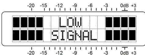
Whenever you go into the 'edit mode'; that is, you enter a menu to make a change to a setup item, front-panel flashing alarms are inhibited while that parameter is being programmed. Menu items that can be edited will 'blink' at a quick rate when the knob is pushed. 'Blinking' menu callouts, as illustrated here, are not to be confused with 'flashing' alarms described above.
