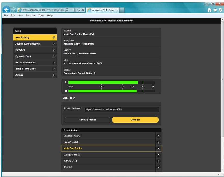
in the Host Name followed by a / (forward slash). Otherwise enter the full IP address of the 610 as shown under Setup / Network / IP Settings. This should take you to the 610's main Webpage, shown here as displayed by Microsoft's Internet Explorer browser.
