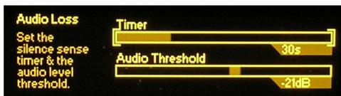
The Timer slider sets the number of seconds between the onset of ‘dead air’ and the alarm. How you set this is dictated by the stream format. A classical music or an oral interpretation stream might call for a setting of 30 seconds or more to allow for the soft passages or long pauses that are native to these formats. A high-energy music channel, on the other hand, could be safe with a 10-second setting.
