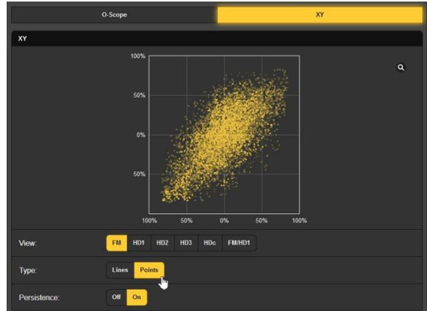
When XY is implemented with a traditional analog oscilloscope, the display resembles a ‘connect-the-dots’ image of the so-named children’s activity. The 551 and most digital ‘scopes can optionally show either Lines or Points. The Points option presents a more artistic ‘constellation’ as seen in the example. In this case Points and Persistence were both engaged to also indicate the short-term trend of the stereo image.
