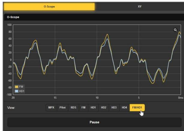
The Pause bar at the bottom of the screen lets you freeze the waveform, and the little magnifying glass in the upper-right corner gives a full-screen display.
